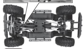
Adjust the slipper by inserting a 7mm hex driver to turn the slipper nut.
